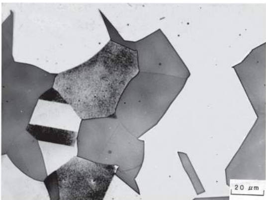
Standard piece No.83 High manganese steel
